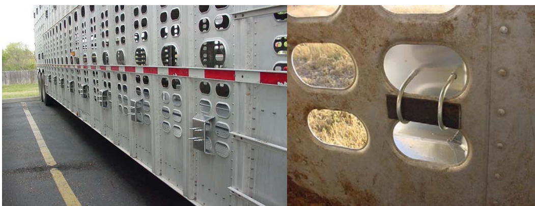
Figure 1. The Wilson scoops mounted to create cross ventilation in the zone between the cattle and the deck. The scoops on the passenger side of the trailer were mounted as intakes on alternate panels while an equal number of scoops on the driver side were reversed to serve as exhaust scoops. The mounting system is visible in the photo on the right. Although the U bolts protrude slightly into the compartments, they are well below the body of the cattle, minimizing the risk of injury to the cattle.
