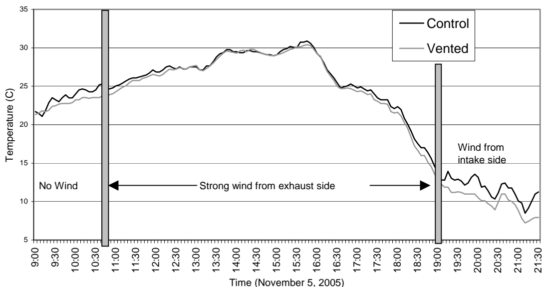
Figure 3. Mean temperatures within the control and vented Wilson cattle trailers during the first trial. The cattle were loaded in Arkansas at 9:00 and unloaded at the Palo Duro Feedyard in Texas at 21:20.
